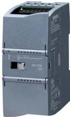
SIMATIC S7-1200, Analog input, SM 1231, 8 AI, +/-10 V, +/-5 V, +/-2.5 V, or 0-20 mA/4-20 mA, 12 bit+sign or (13 bit ADC)
