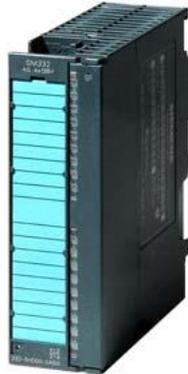
SIMATIC S7-300, Analog output SM 332, isolated, 8 AO, U/I; diagnostics; resolution 11/12 bits, 40-pole, removing and inserting possible with active backplane bus
