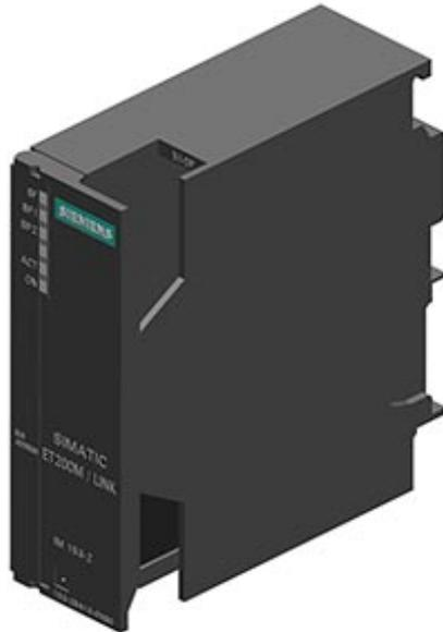
SIMATIC DP, Connection ET 200M IM 153-2 High Feature for max. 12 S7-300 modules with redundancy capability, Timestamping suitable for isochronous mode New features: up to 12 modules can be used Slave INITIATIVE for Drive ES and Switch ES Expanded quantity structure for HART auxiliary variables Operation of the 64-channel modules 32 signals/slot +++Observe compatibility notes in manual+++
