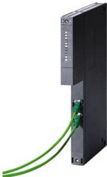
COMMUNICATIONSPROCESSOR CP443-1 FOR CONNECTING SIMATIC S7-400 TO INDUST. ETHERN. VIA ISO, TCP/IP AND UDP, S7-COMM., FETCH/WRITE, SEND/RCV WITH AND W/O RFC1006, MULTICAST, PROFINET IO- CONTROLLER, DHCP, SNMP V2, WEB-, DIAGNOS., INITIALISATION VIA LAN, ACCESS PROTECTION VIA IP-ACCESS LIST, INTEGRATED REAL-TIME SWITCH ERTEC 400, 2XRJ45 CONNECT. FOR LAN WITH 10/100 MBIT/S
