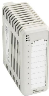
The AI810 Analog Input Module has 8 channels. Each channel can be either a voltage or current input. The current input is able to handle a short circuit to the transmitter supply at least 30 V d.c without damage. Current limiting is performed with a PTC resistor. The input resistance of the current input is 250 ohm, PTC included.
